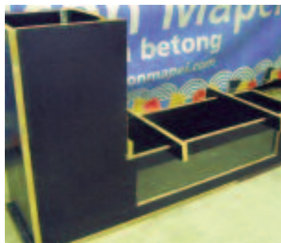
L-box for testing Rescon T
