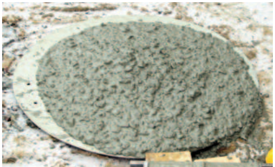
Good workability t-concrete: slump flow > 550 mm
